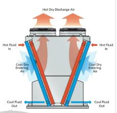
Cooling systems are the thirstiest users of water in many industries like power generation. To defy water dependence and secure sustainable power generation, the acceptance of dry cooling systems in newly built power plants is getting traction. In existing plants built with wet cooling, conversion to hybrid or to dry cooling is also a feasible solution.
